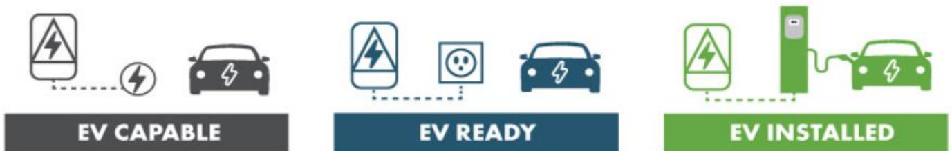
Figure 7.1 EVSE Make-Ready and Building Code Concepts. Source [189]
