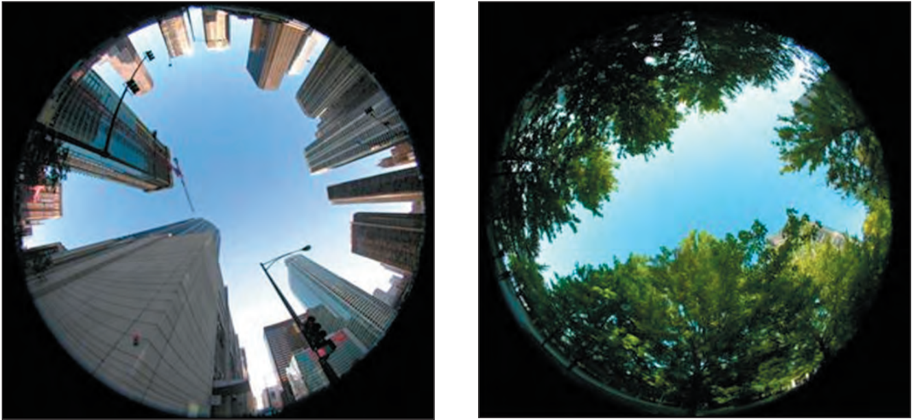
Figure 2-7. Two views from different surfaces that have similar sky view factors resulting from completely different surroundings, one an urban canopy and the other a forest. Photo courtesy of the National Center of Excellence, Arizona State University
