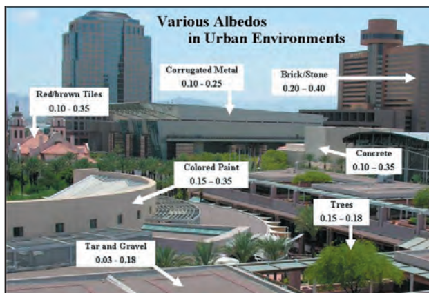
Figure 2-10. A typical urban area, with roof and wall albedo ranges indicated on the different surfaces.
