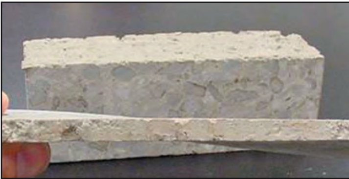
Figure 3-73. Example of a light colored synthetic binder using reflective aggregate. Photo courtesy of the Asphalt Pavement Alliance.
