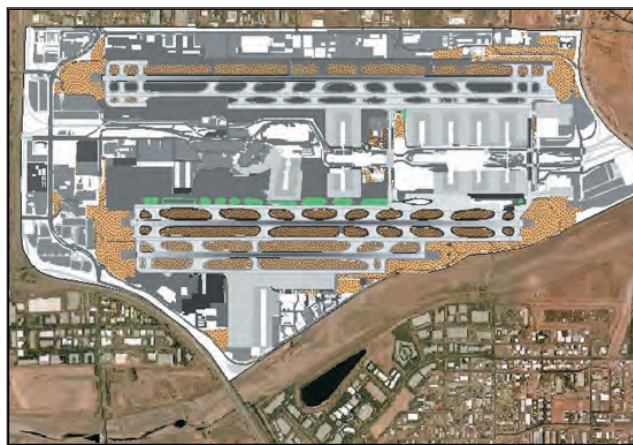
Figure 2-4. GIS image of (a) landscape and bare soil; (b) paved areas within Sky Harbor Airport. (Carlson 2006)
