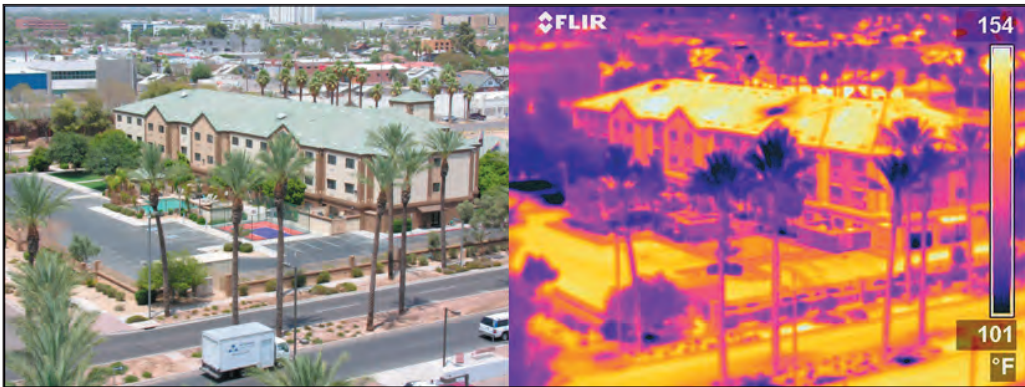
Figure 2-24. Temperature response of roofs, pavements, and walls during an average summer day in Phoenix. Photos courtesy of National Center of Excellence, Arizona State University
