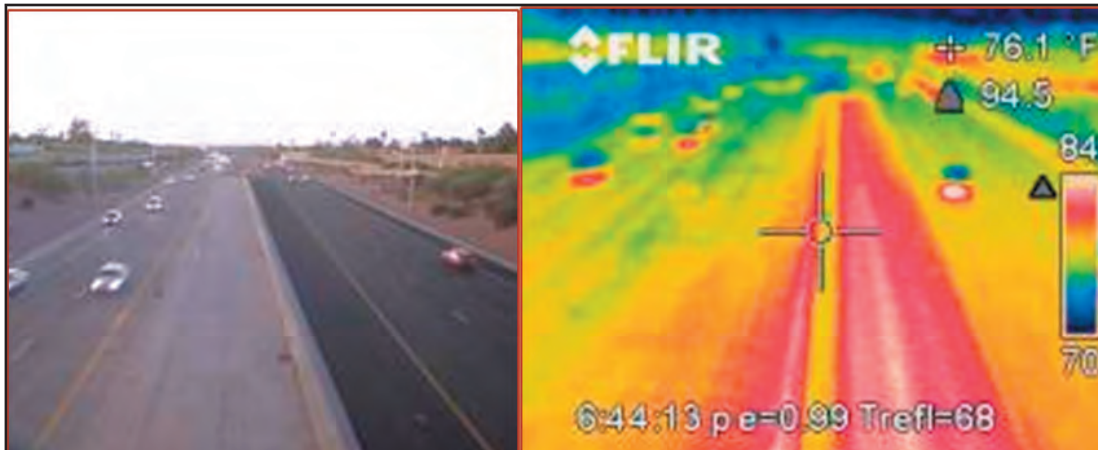
Figure 2-67. Despite its low albedo, crumb-rubber friction course overlays may stay at the same temperatures as Portland-cement concrete in areas of high traffic volume due to convection at the surface. Areas without traffic, such as the highway shoulder in this image, still reach comparatively warmer temperatures during the day. Images courtesy of National Center of Excellence, Arizona State University.
