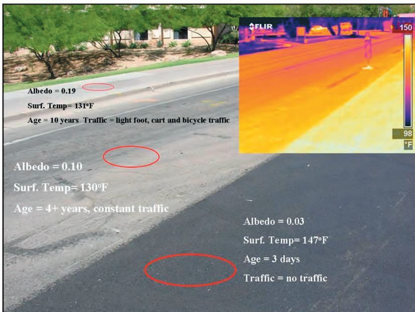
Figure 2-62. New and old asphalt surfaces in the Valley. Courtesy of National Center of Excellence, Arizona State University.
